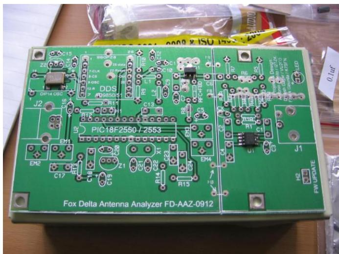
*The PCB is good quality with marking both sides and plated through holes. Surface mount components are already mounted. Note the separate earth plane for the RF section of the analyser board.*
