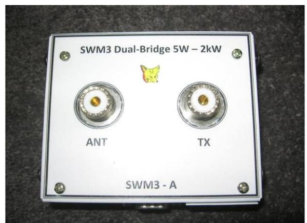
*The dual 200W / 2kW measurement bridge*
